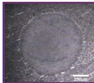
At left is a 1 mm crater in NIST 610 glass. With the UP266MACRO, 266nm, short UV ablation has broken the 1000 µm barrier.
