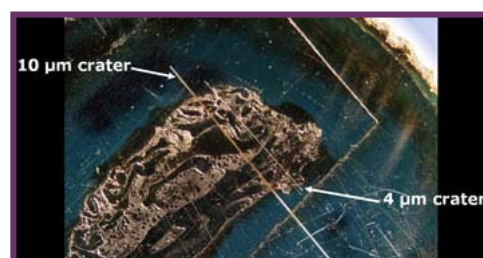
Figure 2: Continuous laser line using a 4 \mu\text{m} and 10 \mu\text{m} crater
