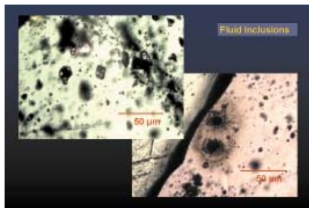
Figure 1: Fluid inclusions in a quartz sample prior to and after the laser ablation.
