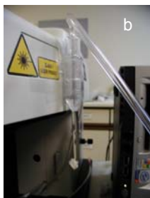
Figure 3: (a) UP-266 MACRO, large beam UV laser ablation system with (b) bubbler, particle filtering device. Schematic diagram of bubbler (c).
